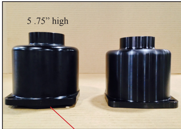
Pilot ring built into hammer case to align with motor housing.
